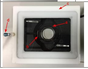
Inset the clamp and dish (a) into the stage by sliding the clamp against the spring plate (b). Place the glass lid on top Attach the tubing to the CO2 aspirator bottle
