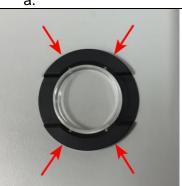
Loosen the screws on the ring clamp and on a flat surface, place the 35mm dish into the clamp. Tighten screws to just hold the dish (DO NOT OVER TIGHTEN).
