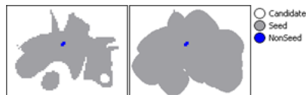
Figure 8.10. Class-based surface tension calculation while growing smooths multiple image objects of a class
