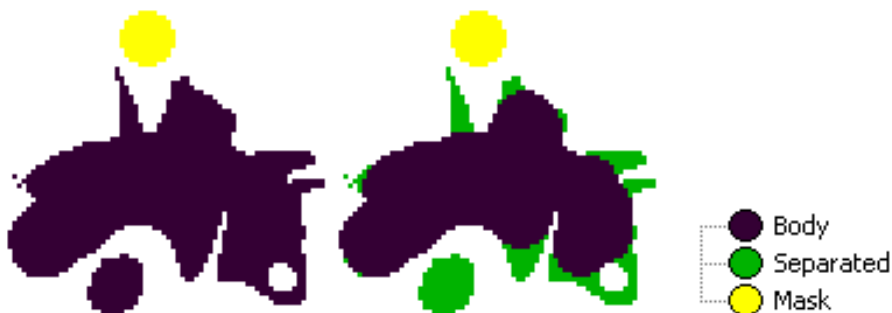
Figure 7.2. Opening operation of the morphology algorithm
