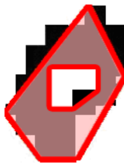
Figure 24.23. A polygon with an inner polygon that is not included in the feature value
