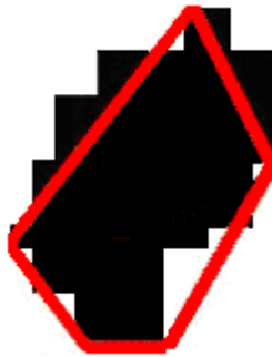
Figure 24.21. Raster image object (black area) with its polygon object (red lines) after vectorization
