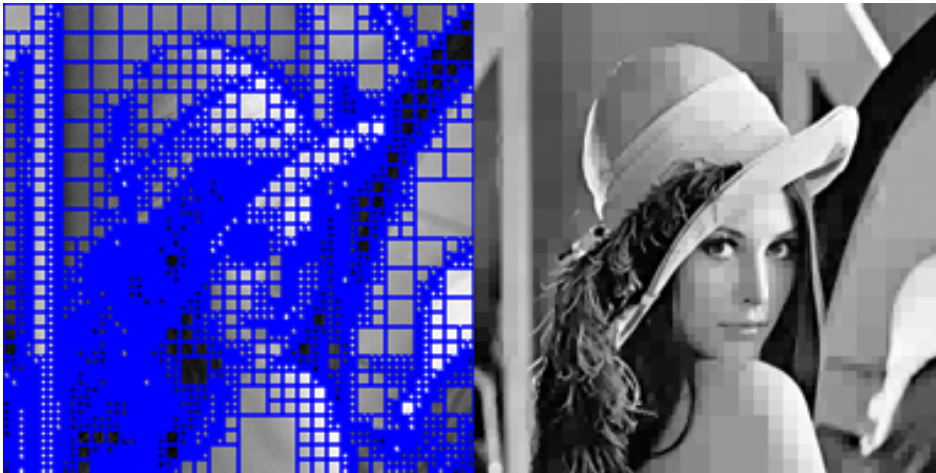
Figure 2.2. Result of quadtree-based segmentation with mode color and scale 40
