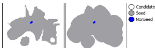
Figure 8.9. Object-based surface tension calculation while growing keeps image objects more separated
