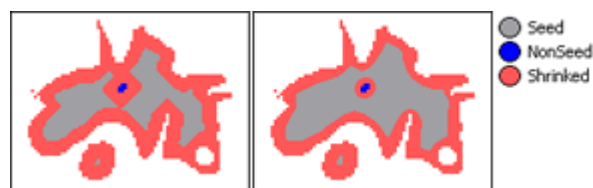
Figure 8.6. Sample classification after 10x shrinking without (left) and with (right) surface tension
