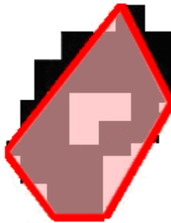
Figure 24.24. A polygon with an inner polygon that is included in the feature value
