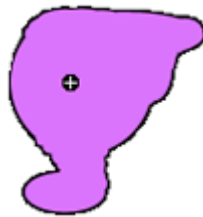
Figure 25.9. Center of gravity of an image object
