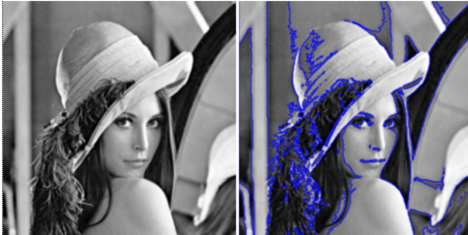
Figure 5.2. Result of multi-threshold segmentation with rule set as described above
