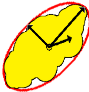
Figure 24.14. Radius of the smallest enclosed ellipse of in image object v , for a 3D image object
