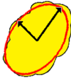
Figure 24.7. Elliptic fit of an image object v
