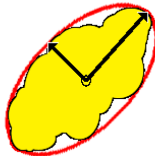
Figure 24.13. Radius of the smallest enclosed ellipse of in image object v , for a 2D image object
