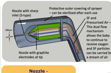
The SF is electrostatically charged as it passes through an electrostatic field produced between the electrode on the front of the nozzle. A sharp inlet is used as opposed to rounder edges to keep the spread of the spray narrow as it is carried by the electromagnetic field through the airway, but still allowing SF to spread out and coat the alveoli as distance increases. This is because the jet from a sharper inlet has minimum breakup while that from a round inlet has a broader spatial
