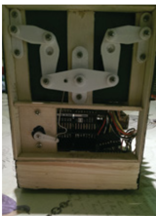
Andy's mechanism showing the Watt's linkages used to approximate straight line movement for Hans and Matilda
