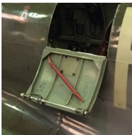
... and then into the cockpit over the door – which you'll notice has a crowbar fitted in case the canopy is stuck and the pilot needs to break their way out in an emergency!
