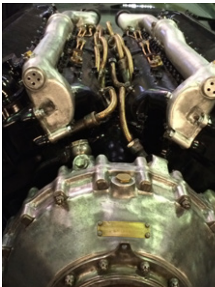
“The Merlin engine is refurbished and zero timed by Retro Track and Air Ltd with the engine bearer manufactured by us here at the Spitfire Company. We then fit the bearer, engine and propeller, at which stage the Spitfire gets to look like a real warbird once again.”
