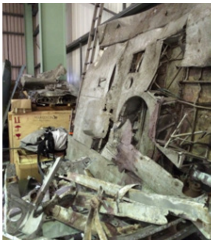
Some Spitfires, like the one above, are in a very sad condition when they first arrive. But as much material as possible is recovered and cleaned up to be reused, keeping as much authenticity as possible.
