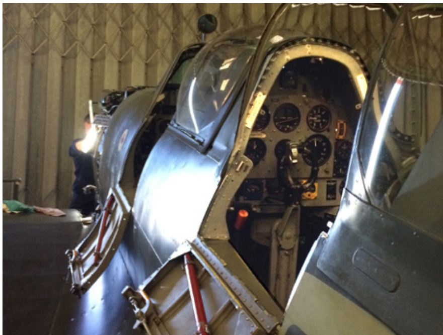
MJ627 was built in 1943 as an LF Mk IX and entered service with the Royal Canadian Air Force in 1944 as 9G-Q. After damage sustained in a forced landing in the Orkneys, she was repaired and stored. Vickers Armstrong converted the airframe into a two-seat TR9 trainer. This involved removing the central fuel tank and moving the cockpit 12 inches forward to make room for the second cockpit. Sold to the Irish Air Corps, she stayed in service until 1960. In private hands after that, and used as a source of spare parts, she was restored in 1993, suffered some damage in 1998, but flew again in 2002. Now owned by the Biggin Hill Heritage Hangar, she is used to offer flights over the Kent countryside.
