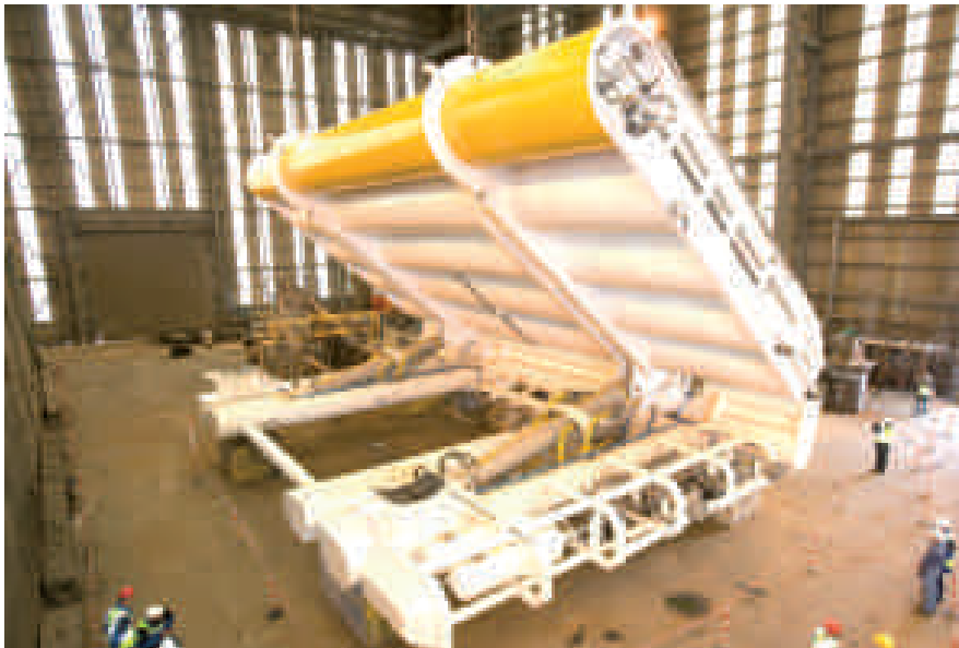
OPPOSITE PAGE: The Oyster hydro-electric wave energy converter is towed into place at EMEC. LEFT: Oyster complete in the factory.
