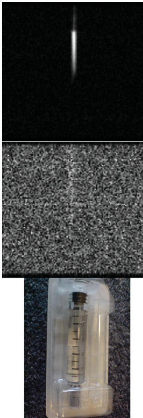
Figure 6 Top: Image of an undiluted Gd-DTPA 10 mL 20 mm diameter, 70 mm length refill tube which has a very short T2* acquired at 3T using TR = 70 ms, TE = 200 \mu s, NEX = 16, in-plane resolution = 1.2 mm \times 0.6 mm, SLT = 2 mm. Image with same acquisition parameters (middle) except TE = 5 ms. The signal from the Gd-DTPA has completely decayed in the later echo time image. The refill tube is pictured (bottom). [Color figure can be viewed in the online issue, which is available at www.interscience.wiley.com .]
