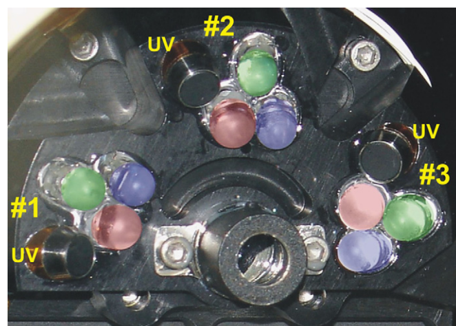
Fig. 1. Front side of the OM. Three clusters (#1, #2, #3) of Light Emitting Diodes (LEDs) obliquely illuminate the target material. The distance from the end of the LEDs to the target is in the range 25–30 mm (Hecht et al., 2008; Goetz et al., 2010a). Each LED cluster is composed of a red (incidence angle i \sim 30^\circ ), blue ( i \sim 30^\circ ), green ( i \sim 37^\circ ), and UV ( i \sim 37^\circ ) LED. The UV LEDs (Nichia NSHU590E, marked in the figure) are covered by a circular UG-11 Schott filter (1 mm thick) on a titanium alloy holder. The circular aperture in the lower part of the image is centered on the optical axis of the instrument and allows a partial view of the lens system. (From Goetz et al., 2010a). (For interpretation of the references to colour in this figure legend, the reader is referred to the web version of this article.)
