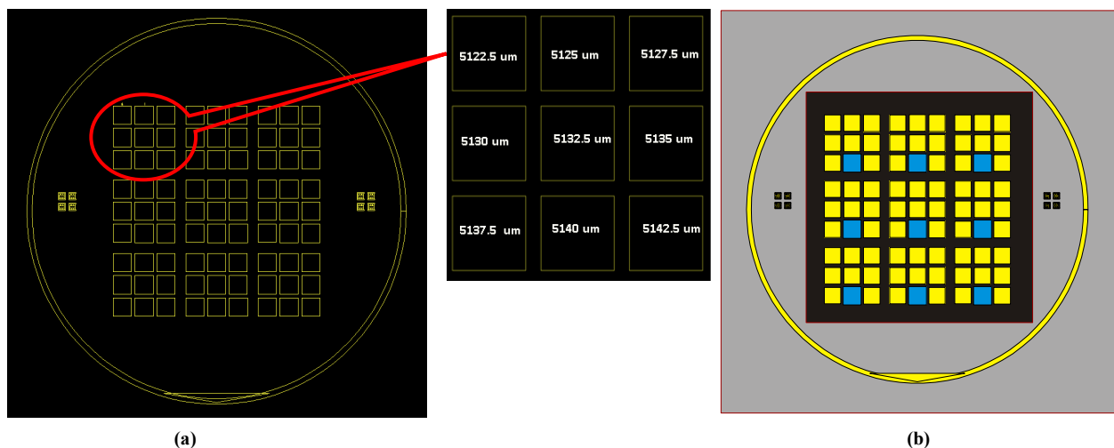
Figure 2. Designs for (a) cavity mask, and (b) selection mask for 5140 \mu\text{m} cavity.
