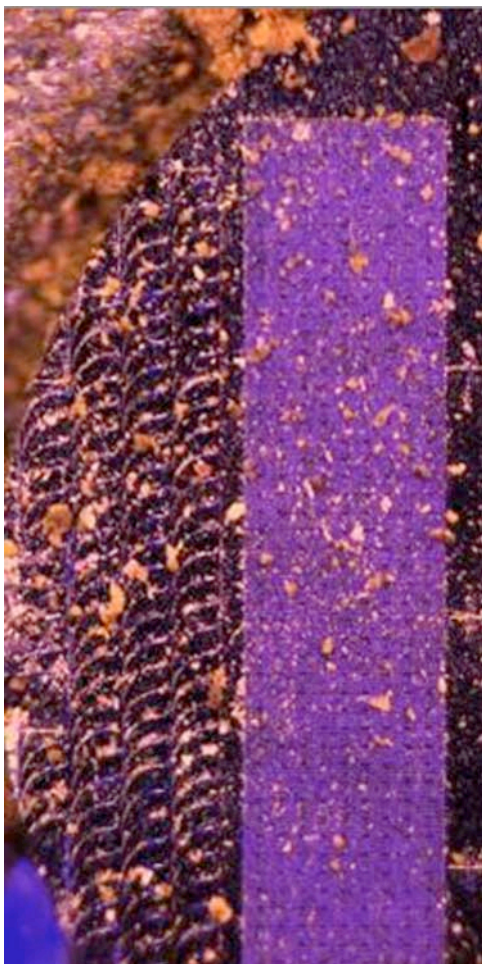
Figure 44. Combined red, green, and blue image of nanobucket substrate acquired on a test bed at Imperial College. The blue object in the lower left corner and the purple band are artifacts of specular reflection from silicon crystal surfaces. The particles, however, are a realistic color and stand out clearly in contrast.
