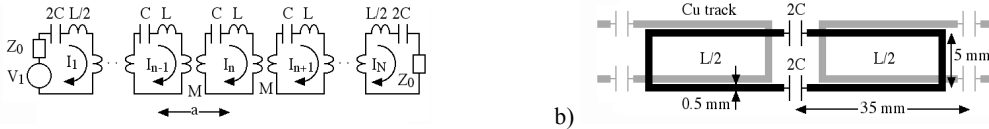
Fig. 1. a) Lumped element circuit for magneto-inductive waveguide, and b) layout of magneto-inductive cable. Assumption of the travelling wave solution I_n = I_0 \exp(-jnk a) , where k is the propagation constant and a is the period, then leads to the dispersion equation:
