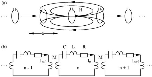
Fig. 1. (a) Magneto-inductive waveguide with nearest-neighbour coupling; (b) equivalent circuit.
