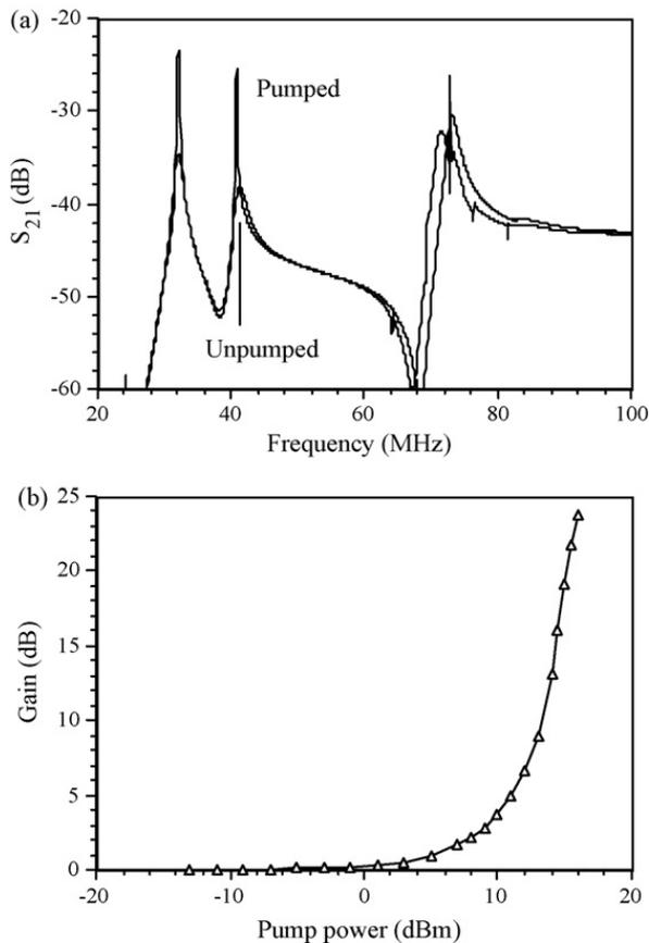
Fig. 6. (a) Transfer characteristics of unit cell, without and with pump applied; (b) variation of gain with pump power.
