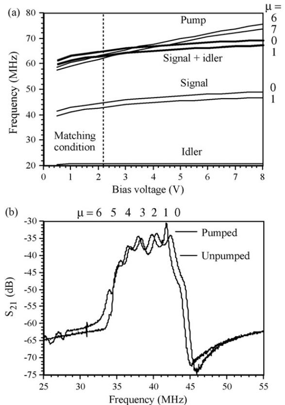
Fig. 9. (a) Voltage dependence of signal, idler and pump resonances; (b) transfer characteristics of ring, without and with pumping by the 6th pump mode to amplify the 1st signal mode.
