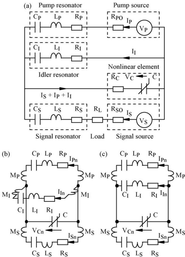
Fig. 3. (a) Three-frequency parametric amplifier; unit cell for amplification of MI waves (b) with and (c) without idler coupling.
