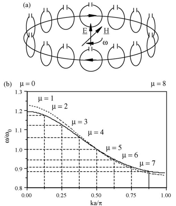
Fig. 2. (a) MI wave ring resonator; (b) MI wave dispersion characteristic, and resonances for a 16-element ring. Full line:  $\kappa_1 = -0.3$ ,  $\kappa_2/\kappa_1 = 0$ . Dashed line:  $\kappa_1 = -0.3$ ,  $\kappa_2/\kappa_1 = 1/9$ .
