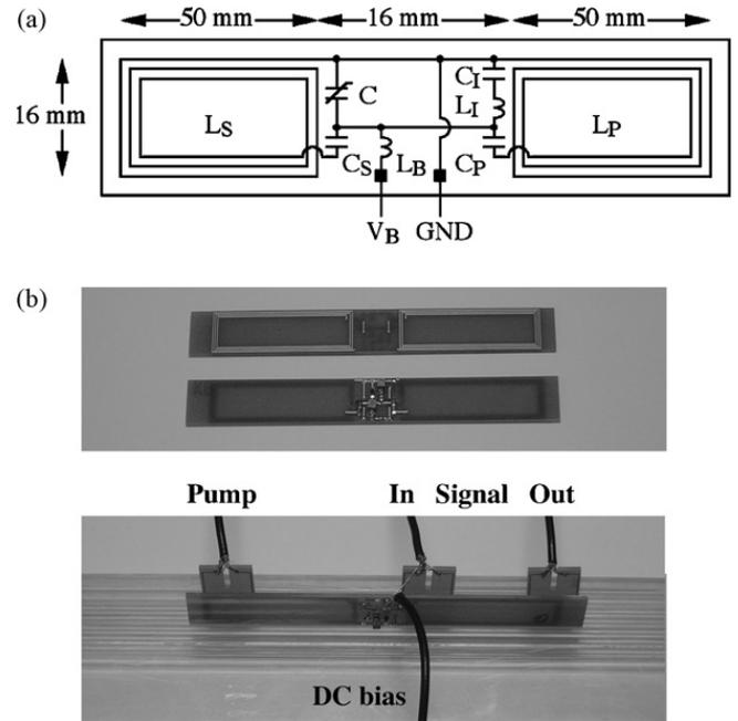
Fig. 4. (a) Layout of amplifier unit cell; (b) prototype unit cell and arrangement for amplification.
