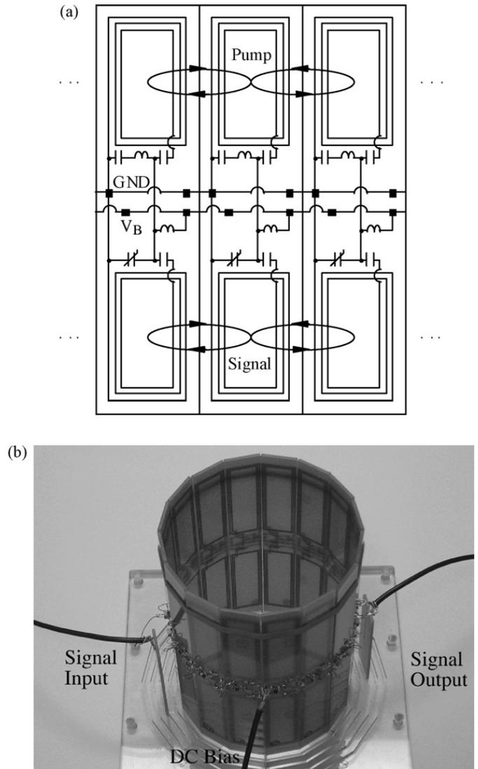
Fig. 7. (a) Arrangement for travelling wave amplification; (b) prototype 16-element ring.
