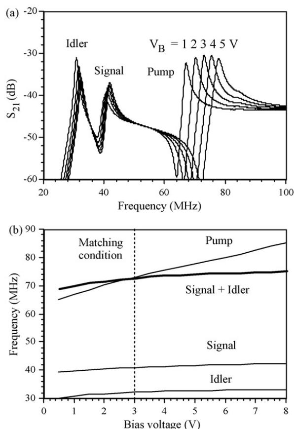
Fig. 5. (a) Transfer characteristics of inductively probed unit cell at different  $V_B$ ; (b) voltage dependence of signal, idler and pump resonances.
