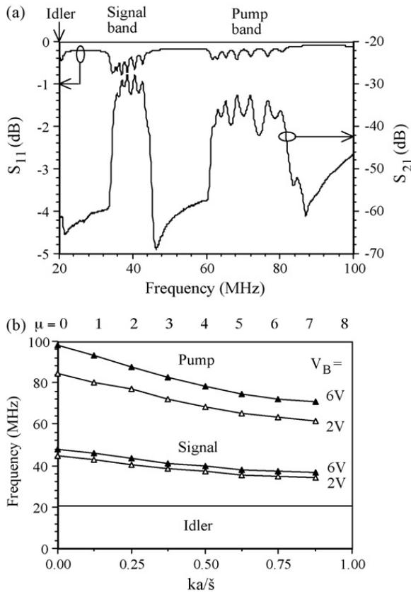
Fig. 8. (a) Transfer characteristic and (b) dispersion characteristic of inductively probed ring.
