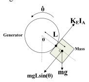
Fig. 1: Schematic of the gravitational torque generator.  $I_A$  is the armature current and  $K_E$  is the motor constant.
