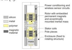
Fig. 10: Schematic of possible microgenerator implementation
