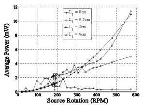
Fig. 9: Average power generated against source rotation at various offset distances,  $l_1$
