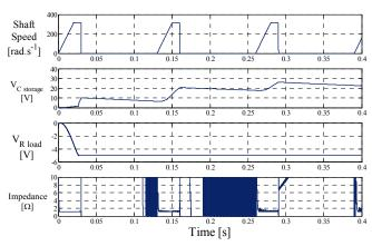
Fig. 7: SPICE simulation results for the model in Fig. 10 with  $R_{Load} = 10k\Omega$  and  $R_A = 1.1\Omega$
