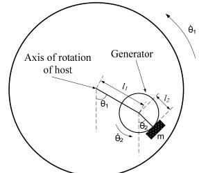
Fig. 8: Schematic of the off-axis generator
