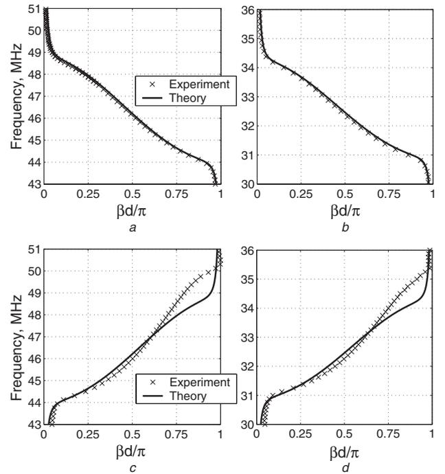
**Fig. 2** Dispersion characteristics of arrays consisting of identical elements
