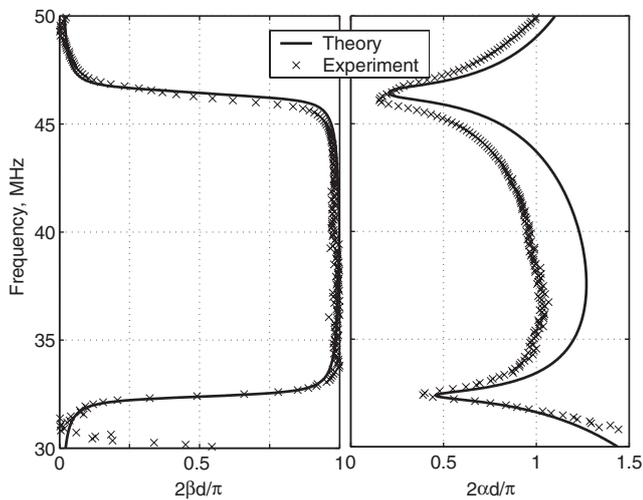
**Fig. 3** Dispersion characteristics for a bi-periodic planar array
