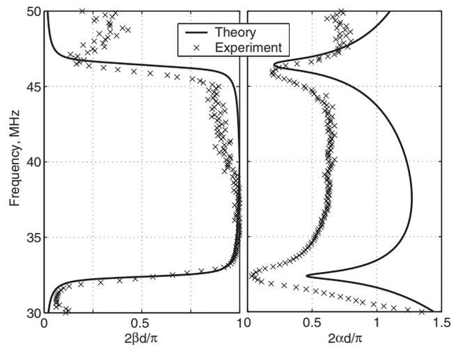
**Fig. 4** Dispersion characteristics for a bi-periodic axial array
