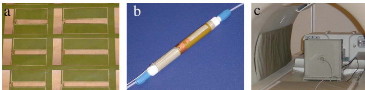
Fig.1: a) Thin film saddle coils, b) coil mounted for testing, c) immersion imaging.
