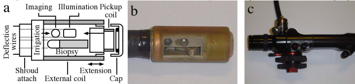
Fig.2: a) Diagram of MR-imaging duodenoscope tip, b) tip, c) handle of MR-imaging duodenoscope
