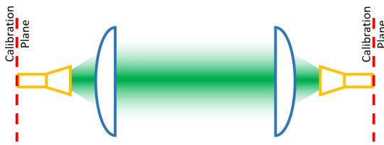
FIGURE 7. Illustration of the limitation for TRL calibration at the VNA's frequency extension heads for our free-space quasi-optical measurement platform.
