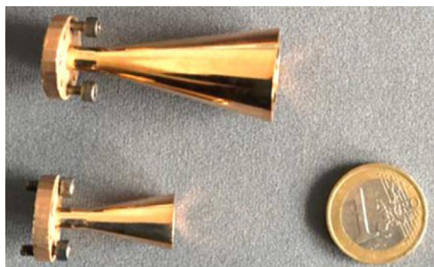
Fig. 6. SLM-printed THz conical horn antennas with MPRWG flanges after postprocessing: D-band (top) and H-band (bottom) [39]. IEEE, reprinted with permission.
