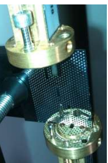
Fig. 2: 100 GHz high Q photonic crystal resonator made from high resistive silicon (from [1])
