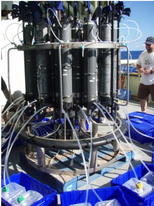
Set up to filter seawater directly from the ship's rosette on the first GEOTRACES intercalibration cruise in June/July 2008.
