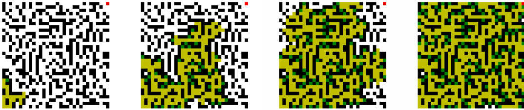
Figure 4.6: Snapshots from BFS algorithm calculating number of dead ends. The green cells represent dead ends discovered. Time moves left to right.
