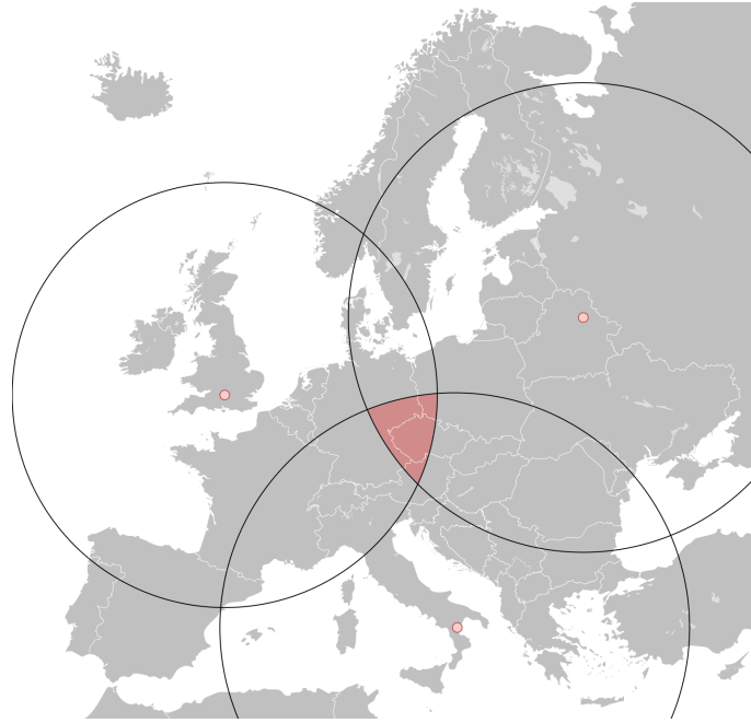
Figure 2.7: Example of performing multilateration using monitors in the UK, Italy and Belarus. The red area shows the range of possible locations of the target.
