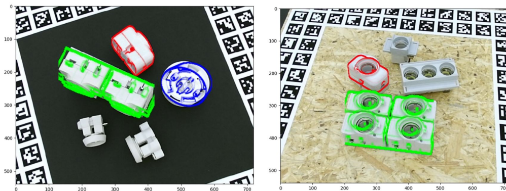
Figure 1.2: 6D pose estimation and object detection using visual cues. Extracted from [18].
