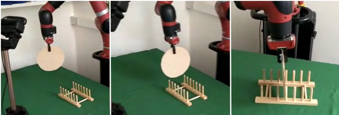
Figure 8.8: Frames from a video of the policy and pose estimator being used on a real robot. The plate should have been placed two slots further right in the rack.
