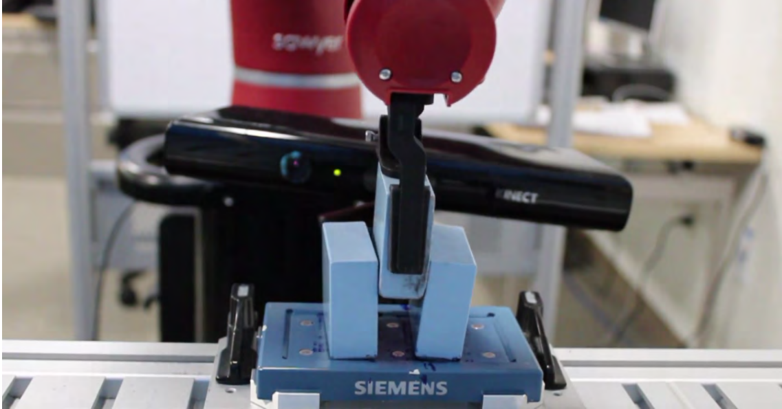
Figure 5.1: A robot attempts to place a block between two others by carefully nudging the other blocks out of the way.
