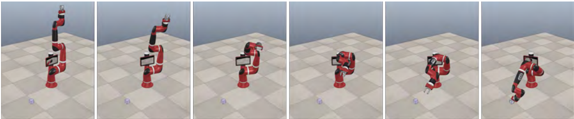
Figure 4.4: Executing the trained Sawyer Reacher policy. The robot travels towards the cube and stops
