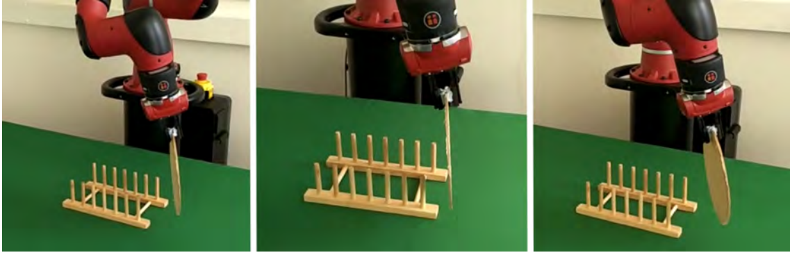
Figure 8.12: End positions of the plate when using the new pose estimator on our strongest simulation policy.
