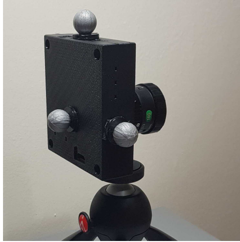
Figure 5.10: Scamp5d device with pearl reflective markers attached to track the position of the device using the Vicon motion capture system.
