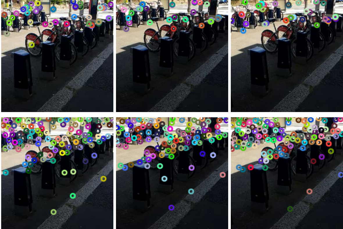
Figure 5.2: Visualisation of the features extracted on the bicycle dataset. The top row is our implementation and bottom row is results from Shi-Tomasi Corner Detector. Our detector fails to detect features in the dark shadowed region of the image.
