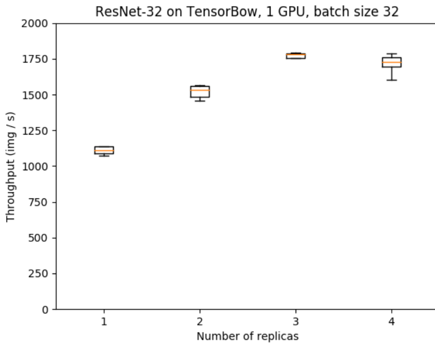
Figure 5.7: TENSORBOW's hardware efficiency when training ResNet-32 on 1 GPU with batch size 32. Beyond 3 model replicas, there is no further improvement in training throughput.
