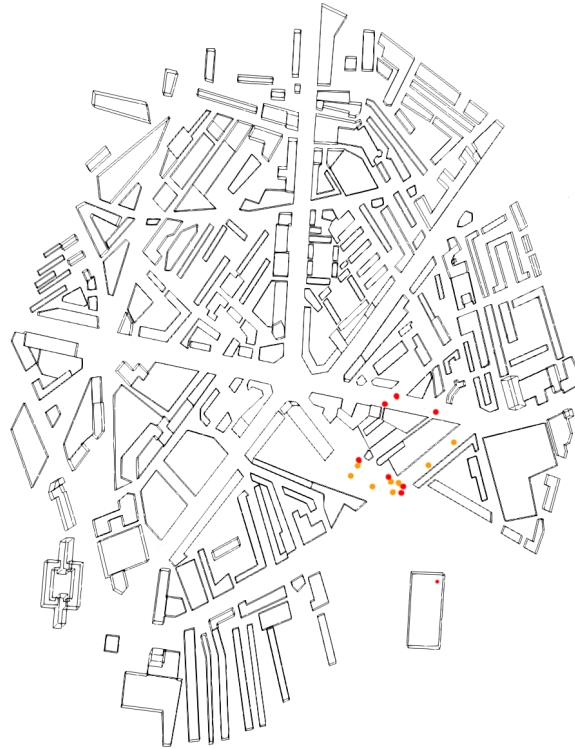
Figure 6.4: Final recommendations for sensor placements in the LSBU test-side. Red: Algorithm 2 Orange: Algorithm 4 (Jitter)
