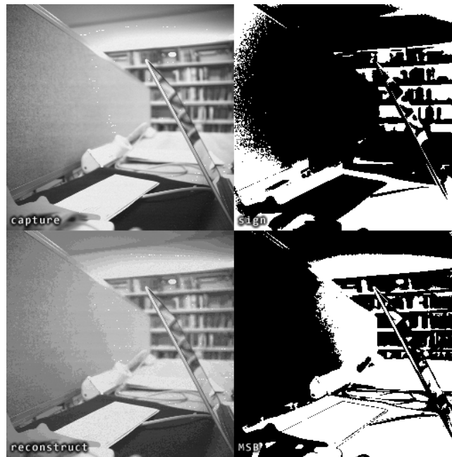
Figure 4.4: Capture of a quantisation on 4 bits processed on the focal plane of the SCAMP5 vision system. Top-left: acquired input image. Top right: DREG storing the sign. Bottom right: DREG storing the first Most Significant Bit. DREGs storing the second and third MSBs are not shown here. Bottom left: reconstructed image.
