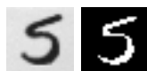
Figure 3.2: Input binarization. Left: original analog image (AREG A). Right: corresponding binarized image (DREG R7).
