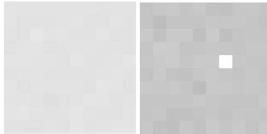
Figure 6.2: Left: crop of 10*10 pixels on a supposedly uniform input value of 100. Right: result after applying our identity kernel 4 times on the input. We can notice a global shift (right image is darker), and an increased amount of noise (right image has more internal variability).
