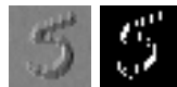
Figure 3.4: Output binarization. Left: result of the first convolution, analog feature map (AREG A). Right: corresponding binarized feature map (DREG R8).
