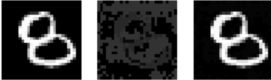
Figure 2.8: Adversarial example found by our algorithm. The image on the left is classified as the digit 8. After adding the noise in the middle (scaled \times 10 to make it visible), the image is classified as a 6.
