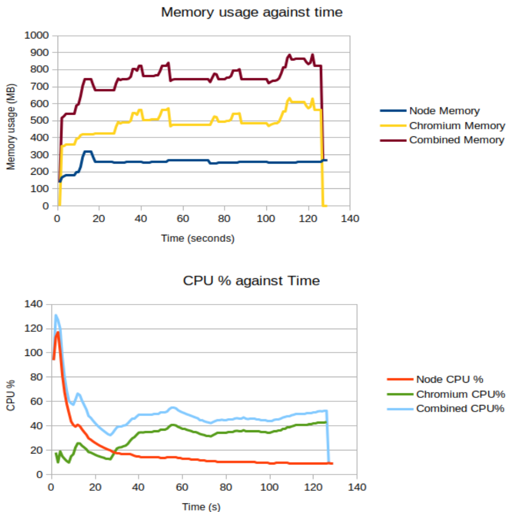
Figure 19: Memory and CPU% statistics while crawling an Amazon phishing page containing three input forms
