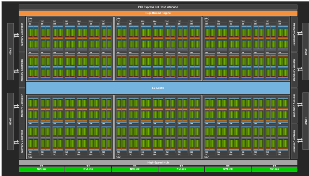
FIGURE 2.2: Architecture diagram for NVIDIA Volta architecture, small green boxes represent arithmetic units. Luke Durant and Olivier Giroux and Mark Harris and Nick Stam, Inside Volta: The World's Most Advanced Data Center GPU , https://devblogs.nvidia.com/inside-volta/ , [Online; accessed January 23rd 2018], 2017.
