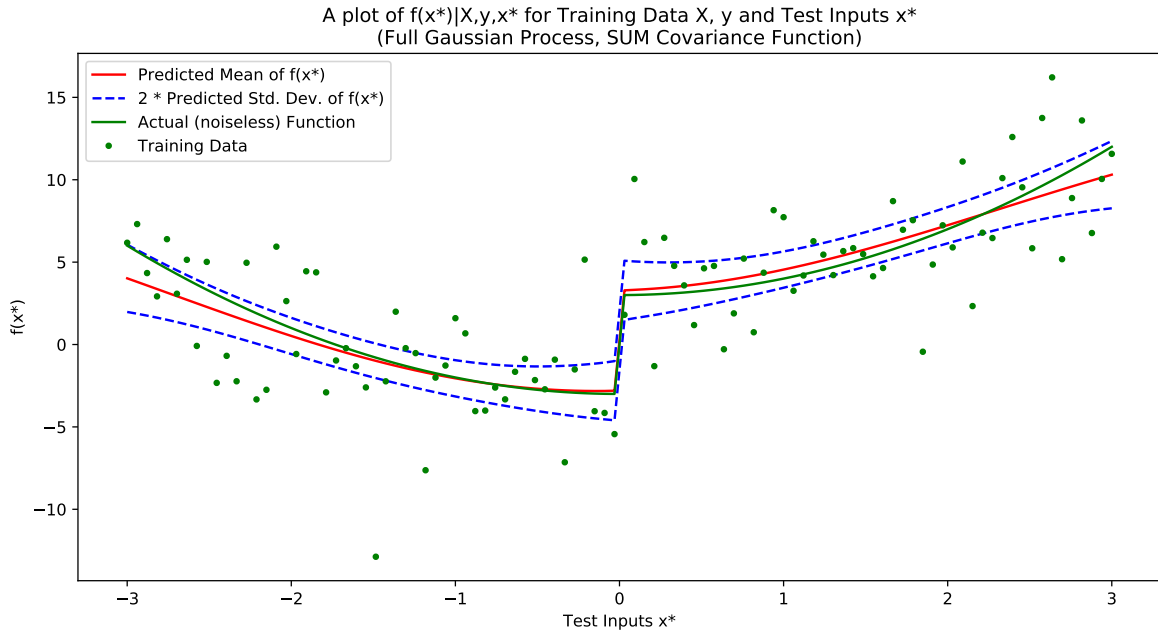
Figure 2.1: Univariate Gaussian process regression with a Rational Quadratic + MLP Kernel and 100 points (x_i, y_i) of training data generated by the system (2.62).
