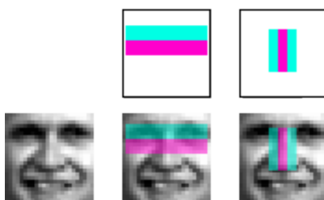
Figure 2.6: Examples of two Haar-Like features applied to a face image. Evaluated feature is the pink sum of pixel values in pink area minus the sum of the pixel values in the blue area. Both features are weak classifiers for a face, with the first one representing the fact that the eye poerion is usually darker than the cheek portion, whereas the other represents a bright nose part with shadows on both sides.
