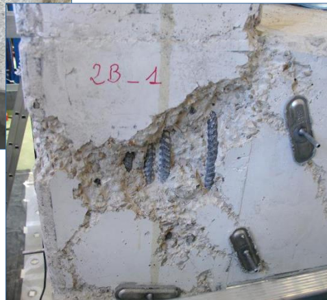
Crack injection, replacement of damaged concrete & surface preparation
