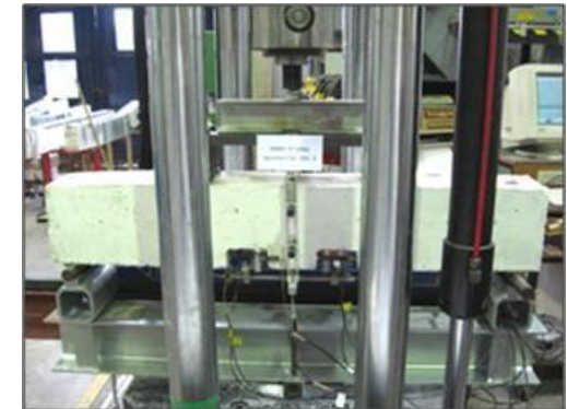
View of beams (Series "S", splice= 10d_b )
