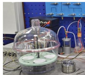
Figure 43. Control of relative humidity in sealed chambers
