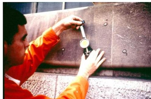
Figure 11. Structural monitoring of cracks with DEMEC Gauge
