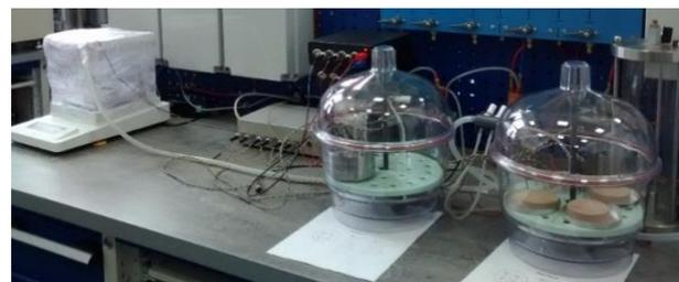
Figure 7. Humidity controlled chambers
