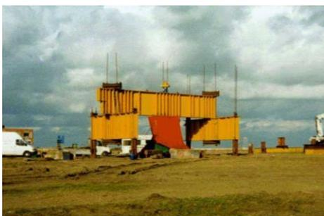
Figure 12. Pile testing at Dunkerque, France
