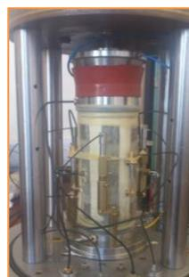
Figure 51. Soil laboratory testing on London clay samples
