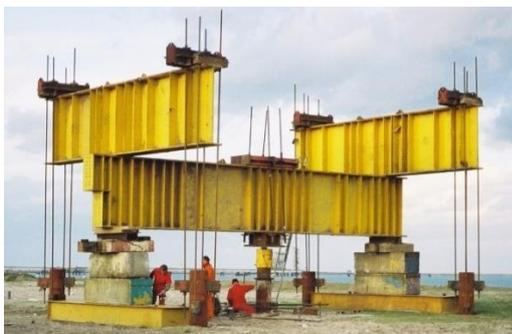
Figure 15. Field testing set up for ICP model pile
