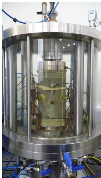
Figure 4. Stress path triaxial testing apparatus, 100mm
