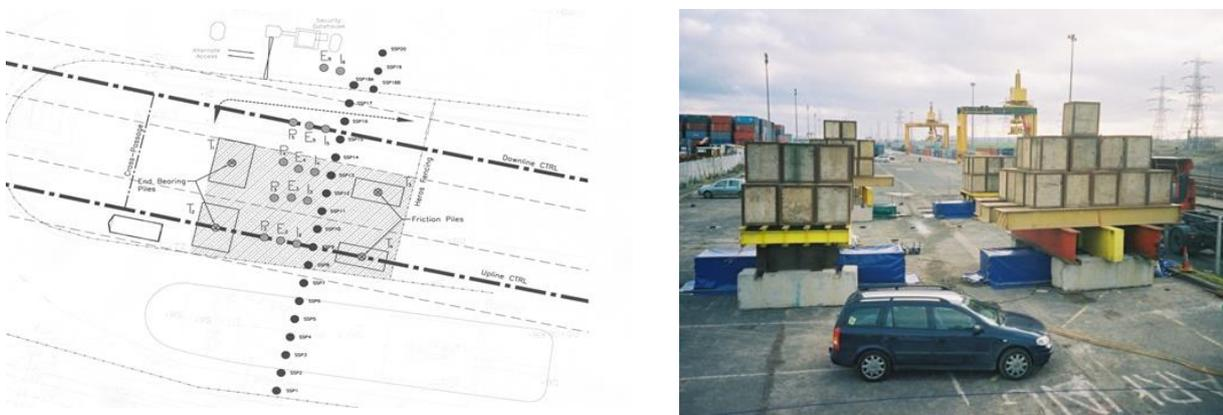
Figure 37. Field monitoring of ground and full-scale pile response to tunnelling in conjunction with Channel Tunnel Rail Link Project (site at Dagenham)
