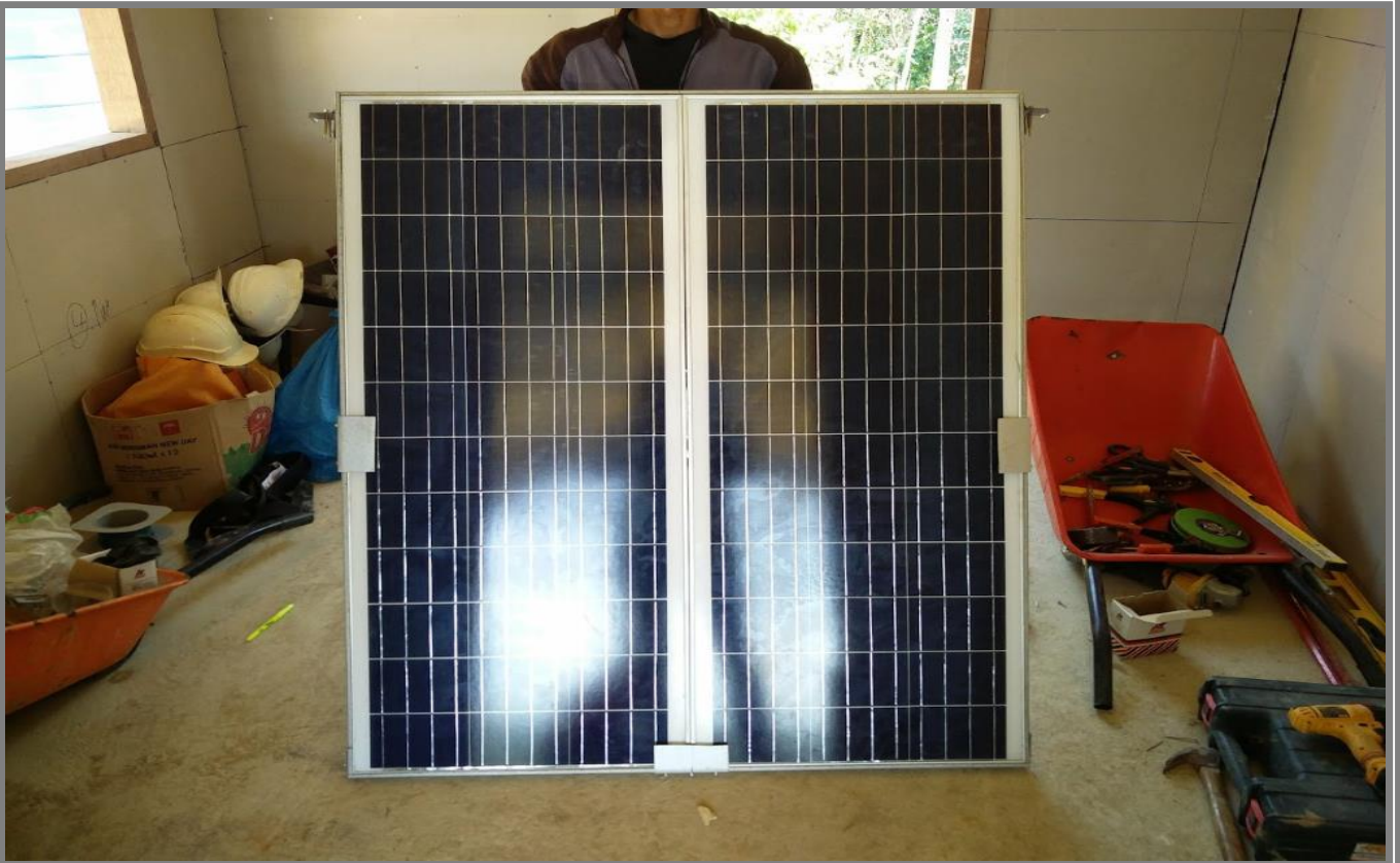
Figure 34: Completed solar panel housing.
