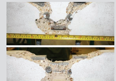
Failure of 3 bar headed bar tension splice.
