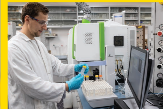
The Roger Perry Laboratory utilises state-of-the-art advanced analytical equipment to enable a fundamental understanding of how elements and compounds behave in the built and natural environment. The ICP-OES (above) is being used to accurately determine, simultaneously, the concentrations of 30 elements in samples of soils collected from contaminated sites.
