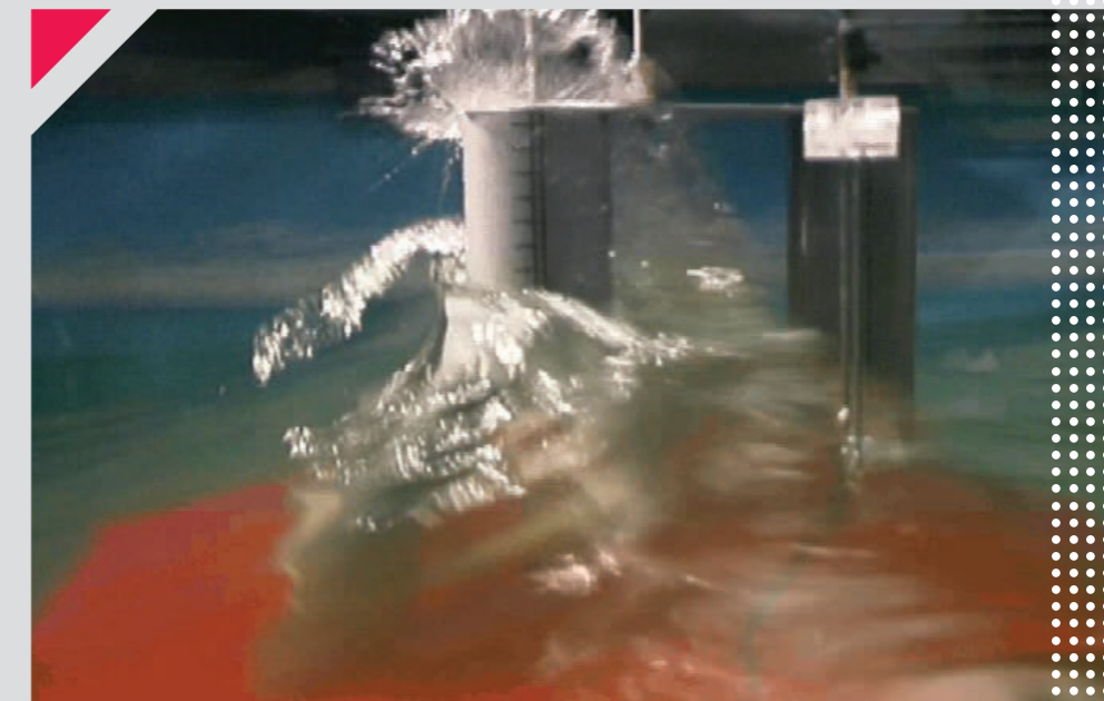
Experimental investigation of wave slamming on a gravity based structure to examine the “ringing” response.
