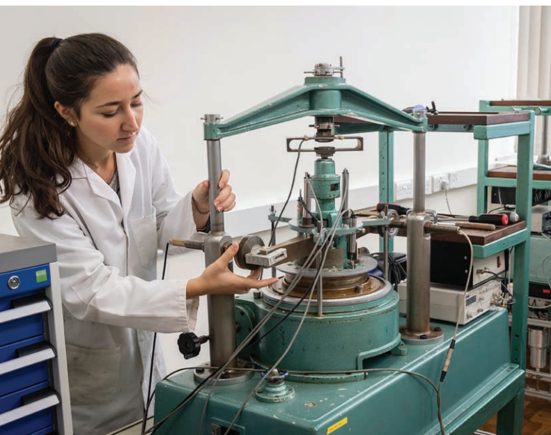
Left: Ring-shear apparatus for determining the residual strength of materials and for characterising soil-pile interfaces.
