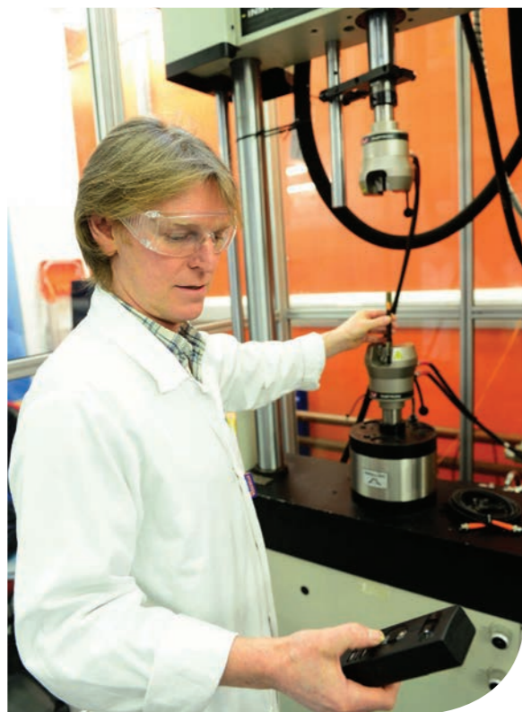
▲ 50 mm single stage gas gun which can fire projectiles between 10–250 g to 60–1400 m/s. ▲ Intron 25kN hydraulic universal test machine is capable of single shot or fatigue testing.
