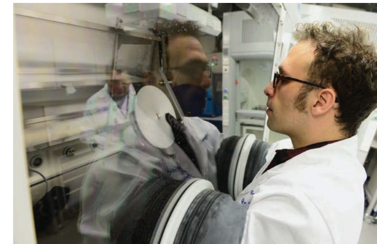
▲ We have glove box facilities to assemble multifunctional structural power materials in a moisture and oxygen free environment.
