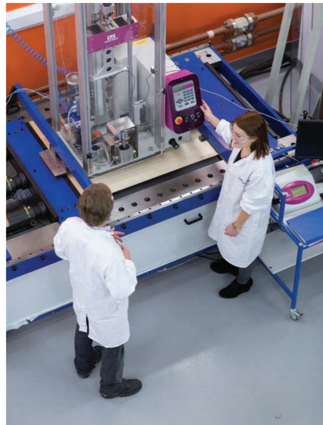
▼ We are investigating the effect of compressive preload on impact resistance of composite structures using our unique impact under load capability.
