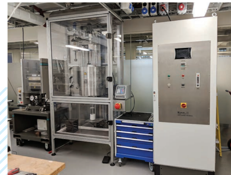
▼ Our furnace for making CNT reinforced light alloys.
