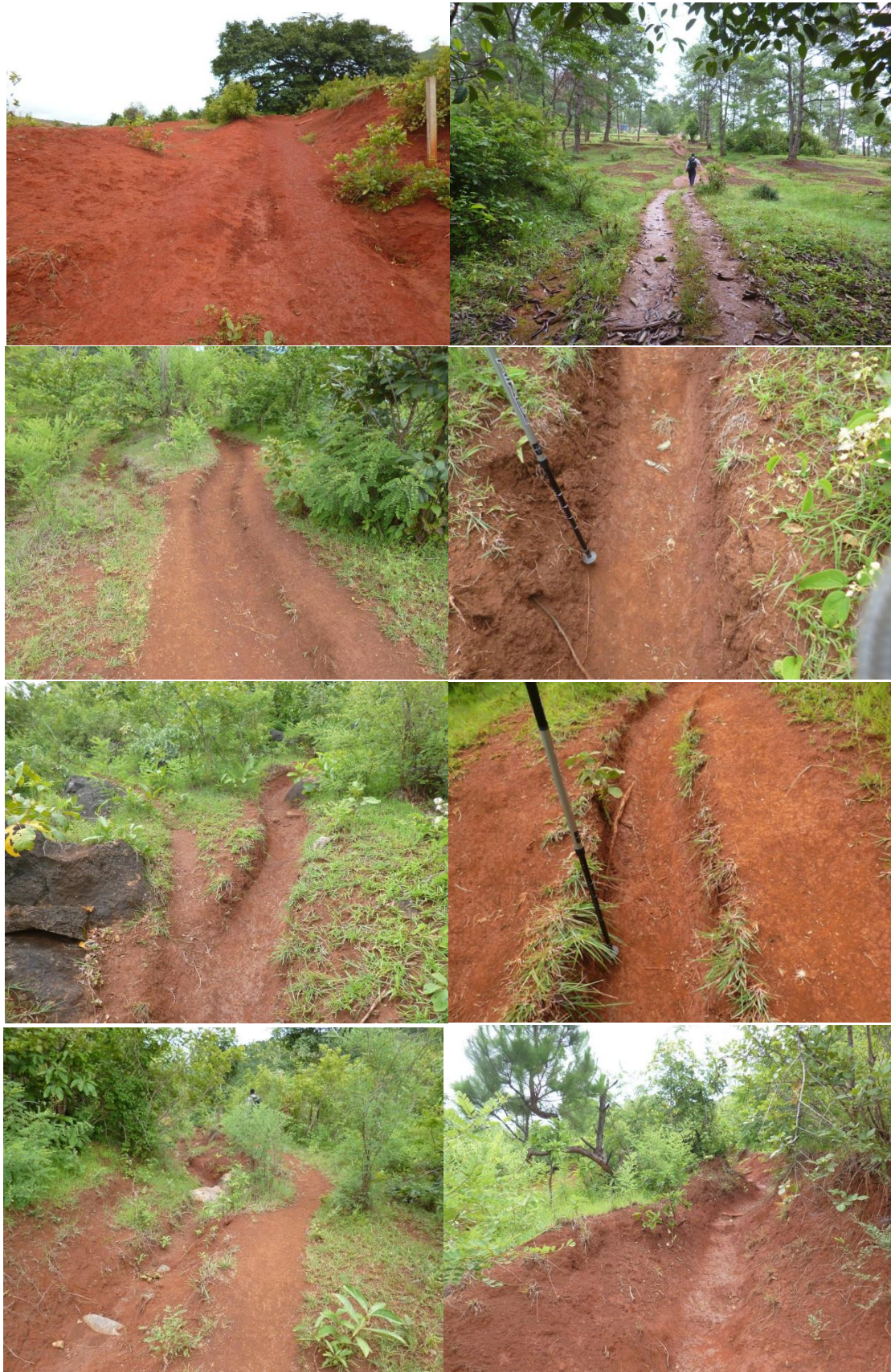
Photographs show the extent of foot path erosion on popular tourist treks. Maximum amount of erosion seen was 0.5 m, average 0.1 m. Footpaths also thought to be eroded by overland flow as part of a run-off drainage network.
