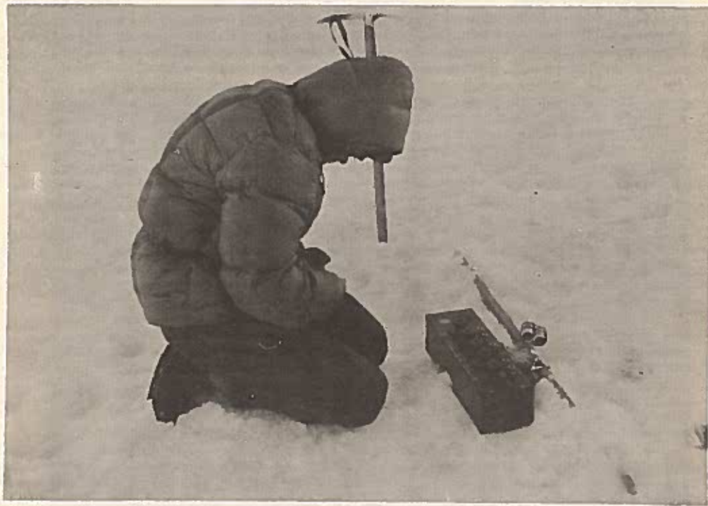
MAKING ELECTRICAL TEMPERATURE MEASUREMENTS OF THE ICE AT DEPTH
