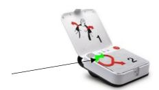
IMPORTANT! DO NOT pull the red handle at this time. Only pull in an emergency. If the red handle is pulled, the electrode seal will be broken, and the electrodes will dry out. If the seal is broken, replace the electrode tray immediately and dispose of the opened electrode tray.
