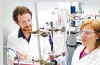
Dr Nick Florin, Research Associate at the Grantham Institute for Climate Change, and Belén González, a visiting PhD student from Instituto Nacional de Estadística, Spain, conducting a precipitation experiment using a slurry bubble column. The overall aim is to be able to remove CO 2 from the exhaust from a large-scale power station, before transporting it to be stored underground.
