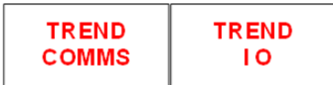
Figure 13 – Labels for BMS field and network cables
