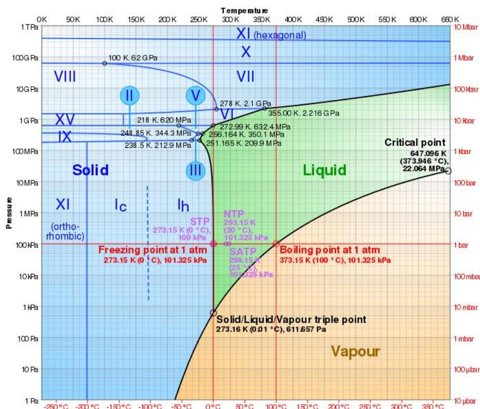
**Figure 2:** Pressure-temperature phase diagram of water.
