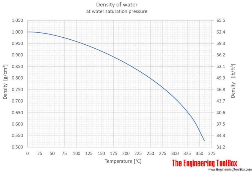
**Figure 3:** Density-temperature diagram of water.
