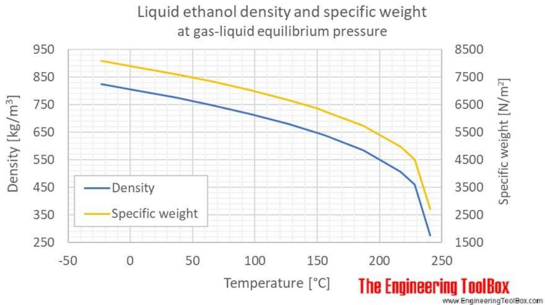
**Figure 5:** Density-temperature diagram of ethanol.
