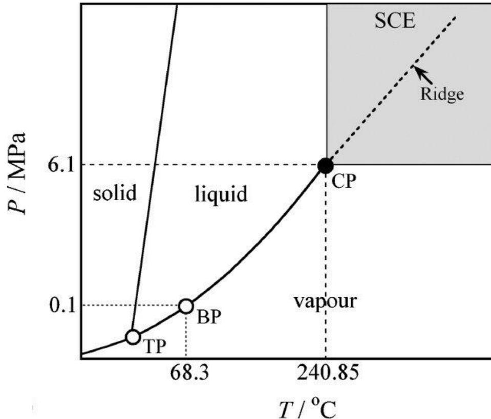
**Figure 4:** Pressure-temperature phase diagram of ethanol.
