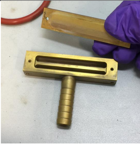
inside the baffle manifold
