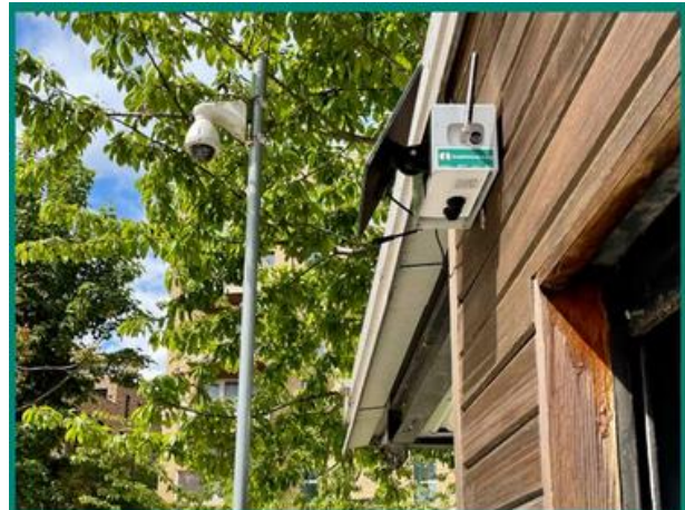
Image: An operational Breathe London node measuring NO 2 and PM 2.5 , powered by a small solar panel.
